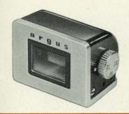
With the viewfinder in place on the camera, you first set the viewfinder for the lens you are using. Turn the "focal length" dial on the left end of the unit (see illustration) so that the correct focal length number ("50," "35," or "100") is opposite the white dot on the viewfinder body. This adjustment, which rotates a system of lenses within the viewfinder, is made only when changing from one lens to another.
