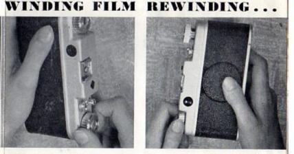
When all pictures have been taken PULL OUT WINDING KNOB and give one-quarter turn to release takeup spool, and rewind film into cassette (using knob marked "rewind" )
