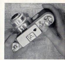
Set exposure counter dial by pushing down and turning clockwise to "0" Turn winding knob as far as it will go. The camera is now ready for the first picture.
