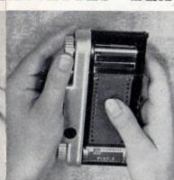
Give the film winding knob a couple of turns to make sure both sprockets engage film perforations.
