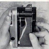
Rotate cradle as shown above to hold film in position so sprockets will engage film perforations.
