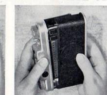
Replace camera back making sure it is securely closed and the catch is in the "closed" position.
