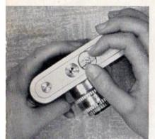
Unlock the back of the camera by turning the catch on the base of the camera to the position marked
