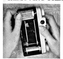
Open and remove back of camera as in loading, and take out cassette.
