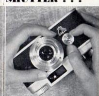
Set shutter speeds (marked in fractions of a second) opposite index dot. DON'T SET BETWEEN NUMBERS. DON'T TURN DIAL CLOCKWISE BEYOND "B", OR COUNTER-CLOCKWISE BEYOND "10"
